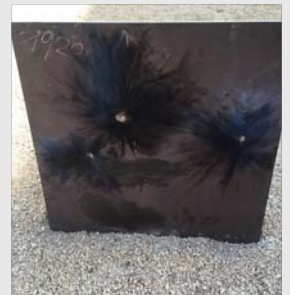
Actual bullet test for armour steel-B7 protection grade
