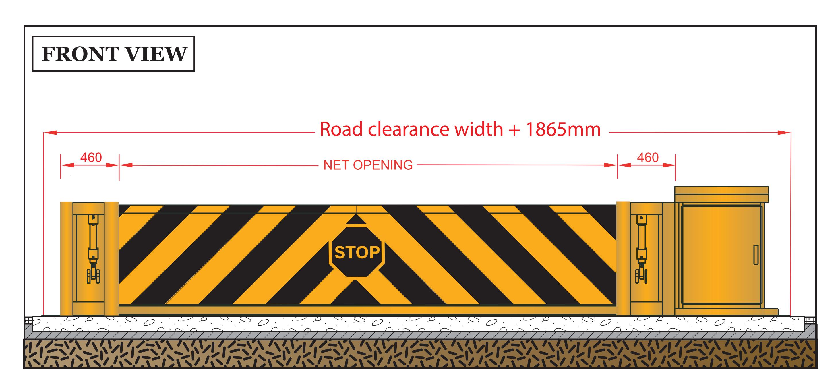
Power unit and hydraulic pistons are attached to the road blocker. Therefore, it increases the road blocker clearance width by 1865mm, It should be considered according to site conditions.
