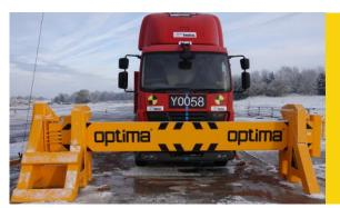
**Crash Test:** PAS68:2013 Gate V/7500(N3)/80/90:0.0/0.0 and IWA14-1:2013 Gate V/7200[N3C]/80/90:0.0 zero penetration.
